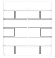
SLEEVE FITS INTO 1 BRICK WIDE BY 2 BRICK HIGH CAVITY Build up brickwork to desired height and set letterbox in place Complete remaining brickwork
